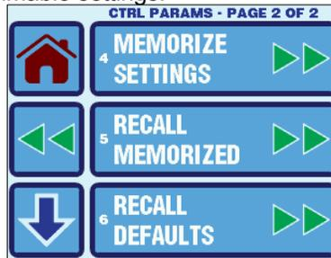
Figure 17- Options to Save or Recall Programmable Settings
