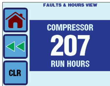
Figure 41- Compressor Run Hours Display
